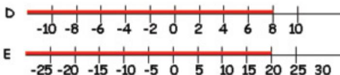
Although the zero on each of these two thermometers is in the same position, and the divisions are the same distance apart, they show very different temperatures. The scale on D is marked in 2s and E in 5s, so although the red lines seem to be the same length, the temperature shown on E ( $20^{\circ}\text{C}$ ) is much higher than that shown on D ( $8^{\circ}\text{C}$ ).
