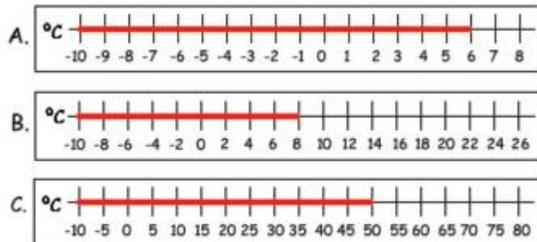
The first thing to do when reading a thermometer is to check the scale. The three thermometers shown above use different scales.
