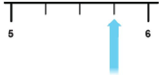
In this scale, the difference between 5 and 6 is 1. The space has been divided into 4, so each mark represents  $1 \div 4 = 0.25$ . The arrow is pointing to  $5 + 0.25 + 0.25 + 0.25 = 5.75$ .
