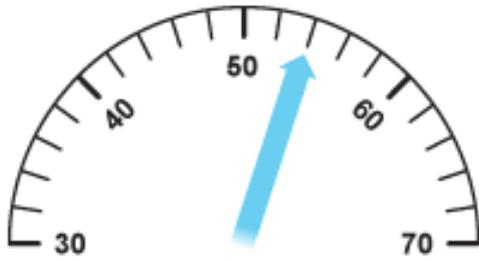
In this scale, the difference between 50 and 60 is 10. The space has been divided into 5, so each mark represents  $10 \div 5 = 2$ . The arrow is pointing to  $50 + 2 + 2 = 54$ .
